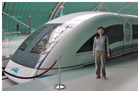
Figure 2: The Maglev train developed in China. This train uses electromagnetic levitation and propulsion to travel, instead of the traditional mechanical method. That means it has no wheels, and is actually floating (or levitating) in the air as it moves!
