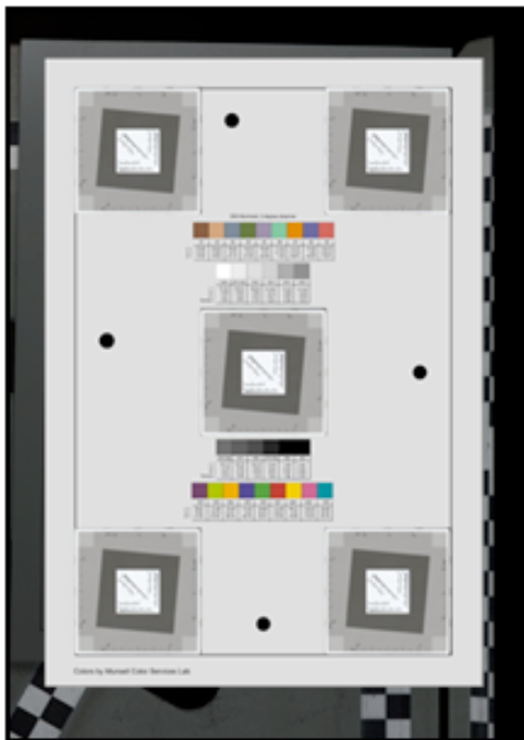
Target used for full Field-of-View Image Quality Analysis "Device-Level Target"
