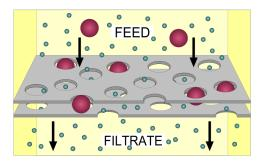
Diagram of simple (dead-end) filtration. http://en.wikipedia.org/wiki/File:FilterDiagram.svg
