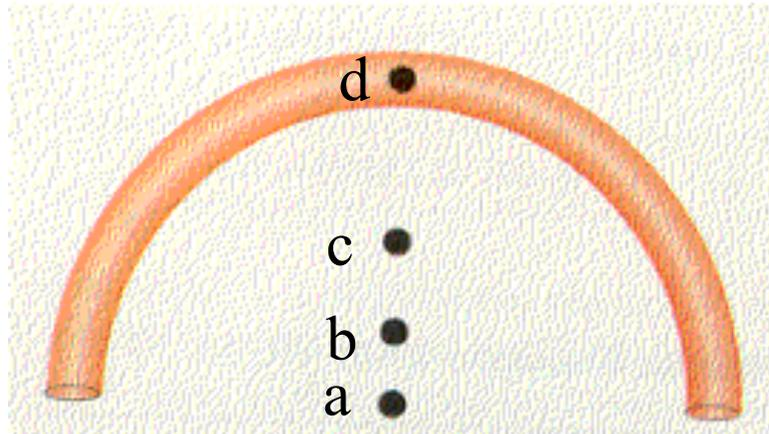
Which point is most likely to be the center of mass of the uniform semi-circular hoop shown?
