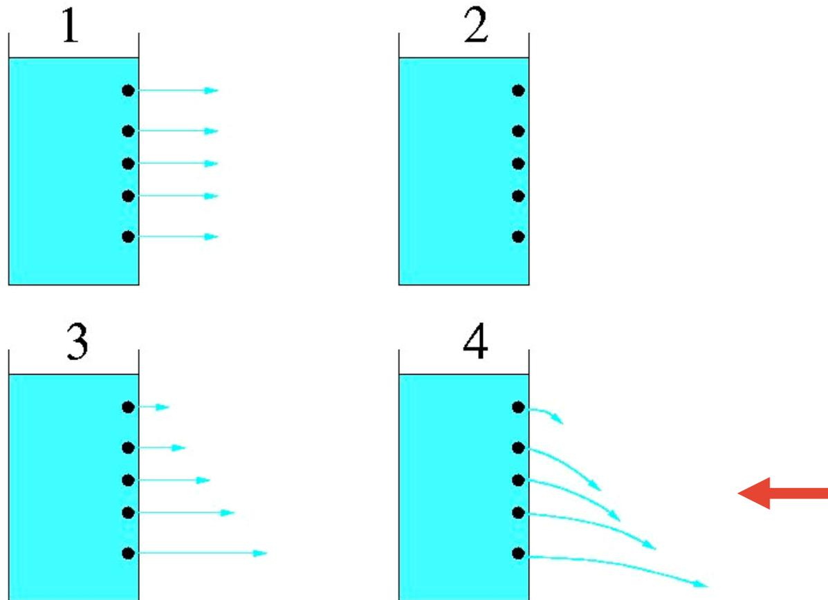
A small water tank with an open top is dropped, preserving its vertical orientation, down an elevator shaft. Just after release, it is rapidly punctured with five, vertically aligned holes. What will resulting flow look like?
